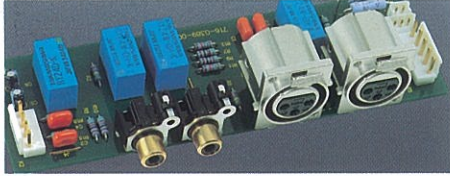
Gold-plated RCA-type jacks and balanced connectors for input
