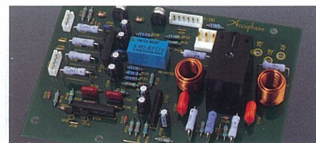
High-current output relays and protection circuit assembly
