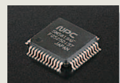
High-speed logic device for DSD → PCM conversion
