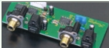
Assembly with transport outputs and digital inputs (optical, coaxial)
