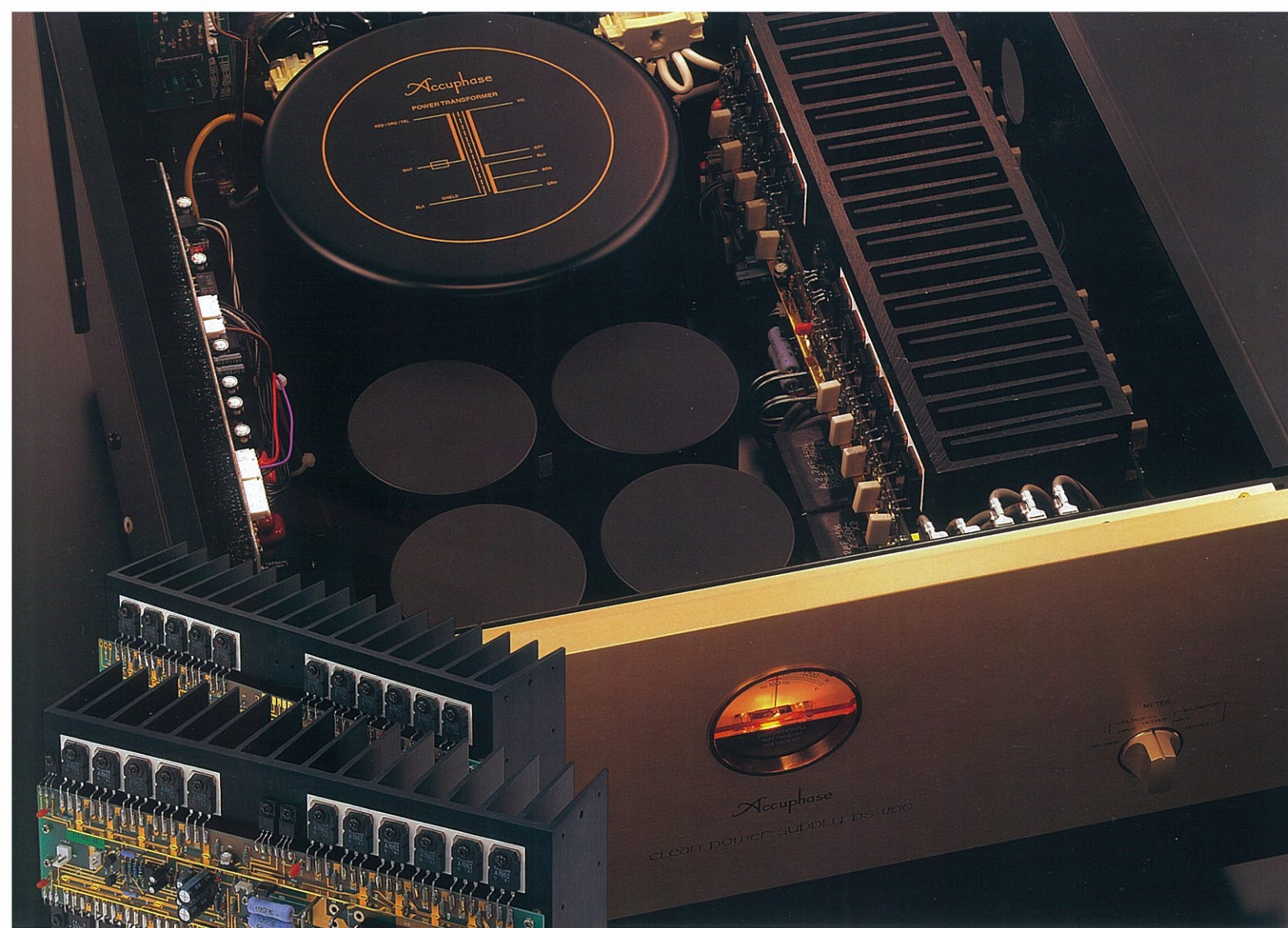
■ Assembly with waveform compensation amplifier for addition/subtraction, output stage with 20-parallel push-pull multi-emitter devices mounted to large heat sink, comparator for reference waveform and output waveform, deviation detector, etc.
