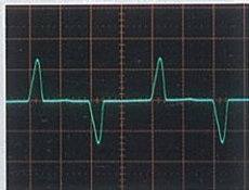
Photo (a) Current waveform of rectified load
