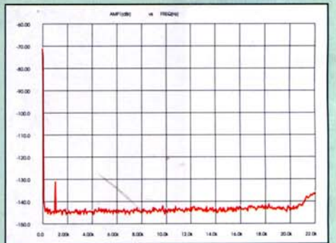
Distorsione armonica (a -130 dB, 1 kHz, banda lineare 0/100 kHz)
