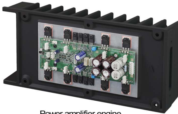
Power amplifier engine
