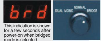
This indication is shown for a few seconds after power-on when bridged mode is selected
