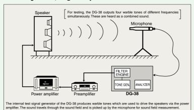
A dedicated sound field measurement microphone with controlled frequency response is supplied with the DG-38.
