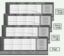
The DG-38 comes with four preprogrammed reference curves: three curves with high-end rolloff (-1 dB, -2 dB, -3 dB per octave) and flat response.
