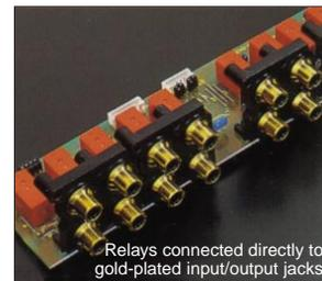
Relays connected directly to gold-plated input/output jacks
