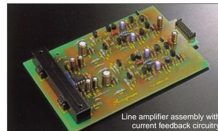
Line amplifier assembly with current feedback circuitry
