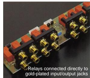
Relays connected directly to gold-plated input/output jacks
