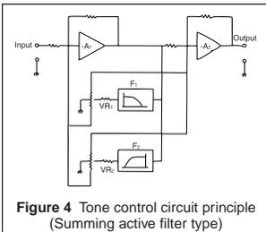
Figure 4 Tone control circuit principle (Summing active filter type)
