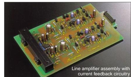
Line amplifier assembly with current feedback circuitry
