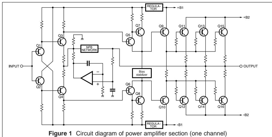
Figure 1 Circuit diagram of power amplifier section (one channel)
