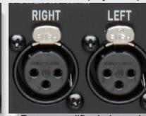
Power amplifier balanced input connectors
