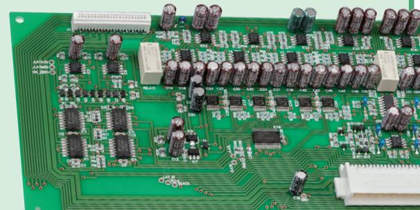
Logic-controlled relays and line input and output connectors
