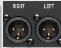
Preamplifier balanced output connectors
