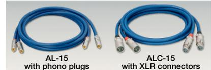
●Type: 2-conductor shielded cable ●Center conductors: [oxygen-free copper wire + silver-plated soft copper wire] ●Jacket: blue PVC, 8.0 mm dia. ●Dielectric: polyethylene + foamed polyethylene ●Total DC loop resistance: 33 m-ohm/m ●Inter-electrode capacitance: 170 pF/m ●Insulation resistance: 40 M ohm/km
