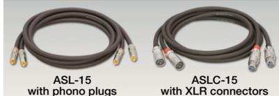
●Type: 8-core multi-hybrid configuration ●Center conductors: high-purity copper wire (7N) + 3 types of copper wire ●Jacket: dark brown PVC, 8.7 mm dia. ●Dielectric: polyethylene ●Total DC loop resistance: 20 m ohm/m ●Capacitance between two center conductors: 378 pF/m ●Insulation resistance: 40 M ohm/km
