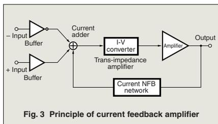
Fig. 3 Principle of current feedback amplifier
