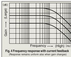
Fig. 4 Frequency response with current feedback (Response remains uniform also when gain changes)
