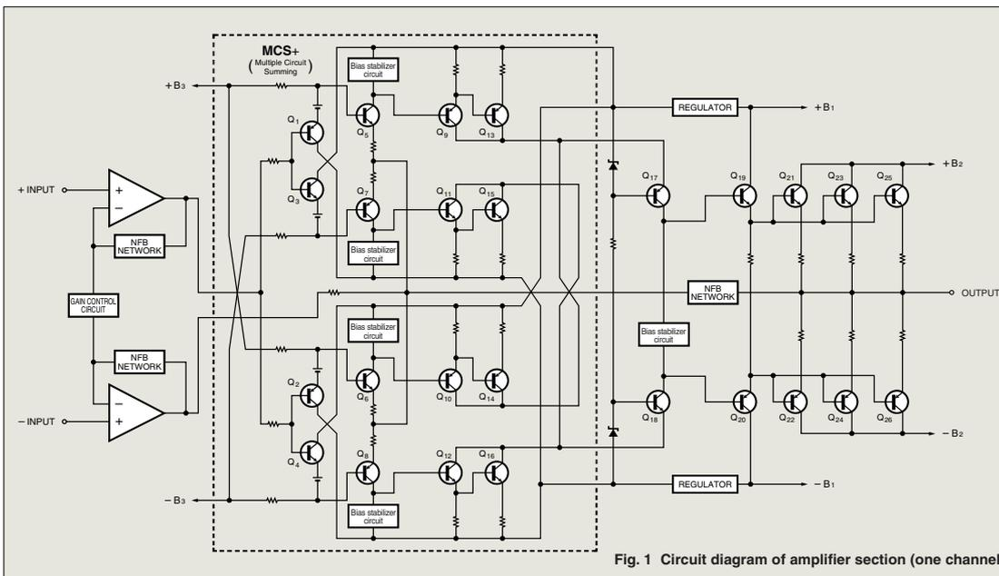
**Fig. 1 Circuit diagram of amplifier section (one channel)**
