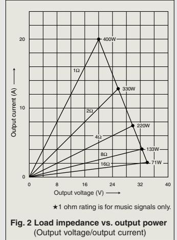
**Fig. 2 Load impedance vs. output power** (Output voltage/output current)
