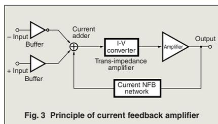
Fig. 3 Principle of current feedback amplifier
