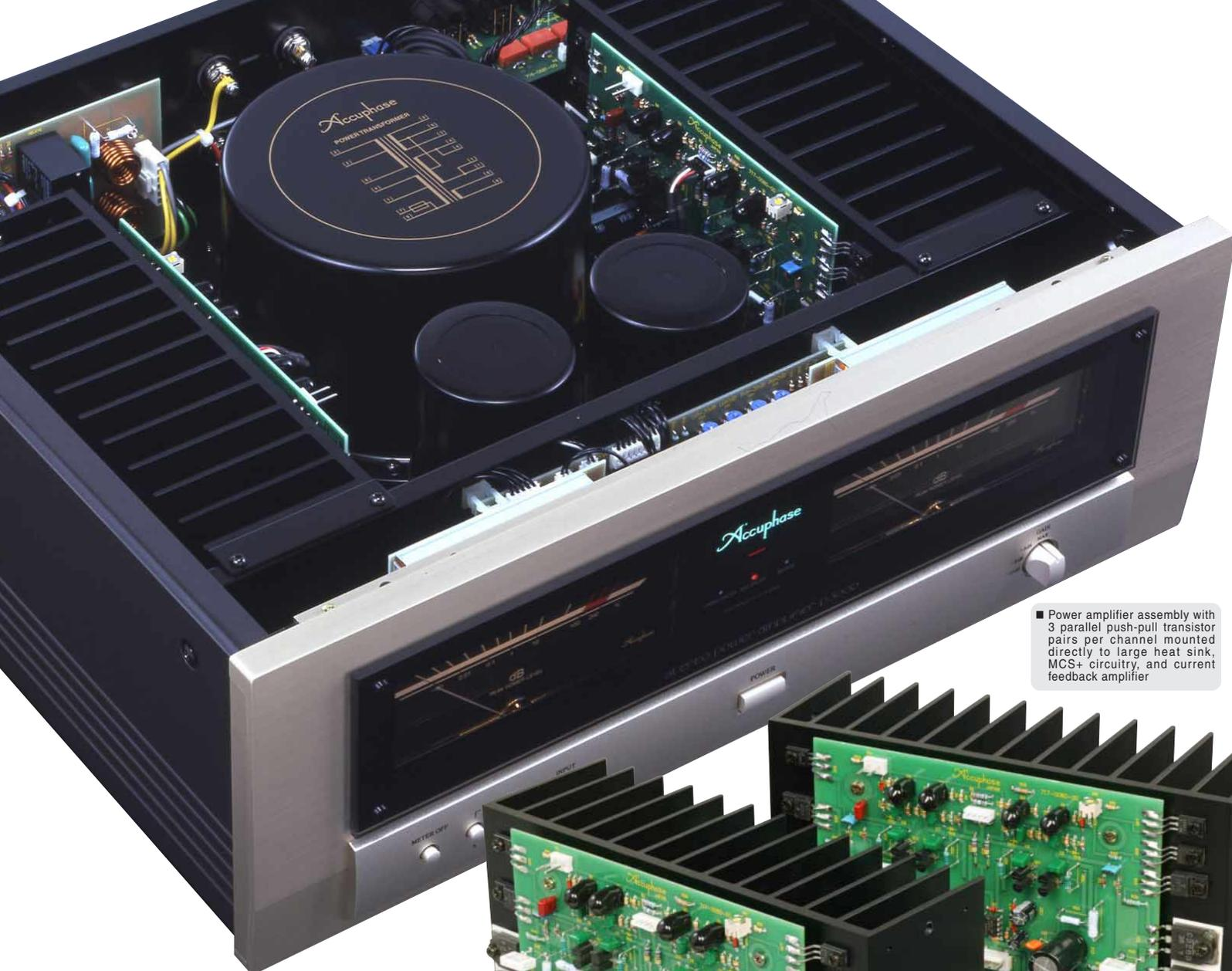
Power amplifier assembly with 3 parallel push-pull transistor pairs per channel mounted directly to large heat sink, MCS+ circuitry, and current feedback amplifier
