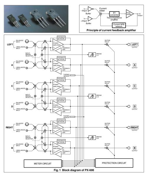
point is kept very low, which means that there is almost no phase shift. Phase compensation via negative feedback can therefore be kept to a minimum, resulting in excellent transient response and superb sonic transparency. Figure 3 shows frequency response for different gain settings of the current feedback amplifier. The graphs demonstrate that response remains uniform over a wide range.
