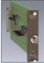
**For BNC coaxial cable input**
