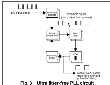
voltage-controlled oscillator (VCO) using a quartz crystal element. The master clock produced by this PLL circuit is totally free from the effects of pulse distortion and jitter.
