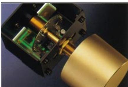
generate a series of pulses in a phase detector. These pulses are utilized by a microprocessor to govern the volume control function. For the user, the volume control of the DC-330 operates with a silky smooth and natural feel that perfectly matches the audible change in volume. The current volume setting is indicated by the numeric display and also by an array of LEDs on the circumference of the control. This lets you check the setting at a glance.
