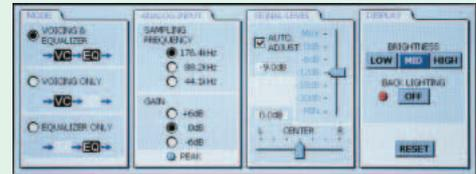
This screen lets you make environment and function settings, such as selecting the Voicing/Equalizer modes, controlling the sampling frequency and gain for the analog inputs, setting output levels and left/right balance, adjusting screen brightness, turning the display on and off, etc.
