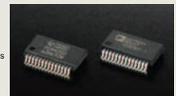
■ High-performance/high-precision delta-sigma A/D converter and D/A converter
