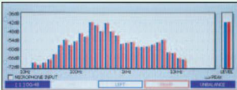
After selecting either L&R or L/R, the content of the input signal can be displayed on a frequency spectrum screen with 1/3 octave spacing, in 35 bands, in real time. It is also possible to check total peak levels, compare the Voicing and Equalizer On/Off conditions, and display the frequency spectrum of the microphone input.
