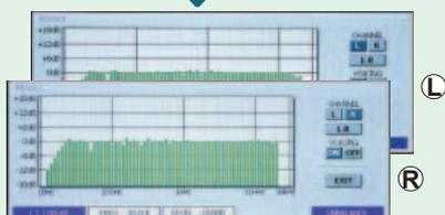
L/R channel characteristics example for performing sound field compensation with the "flat" target curve. Peaks and dips caused by listening room acoustics and speaker characteristics are evened out, resulting in approximately flat response.
