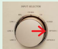
Installation example DAC-30 installed in rear-panel option board slot, input selector set to "OPTION 1"
