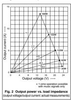
current characteristics for various load impedances. Output voltage remains largely
