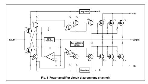
constant even when load impedance changes, which means that the current increases linearly. The amplifier has ample reserves to handle musical signals with transient pulses, which is demonstrated by the clipping power rating from actual measurements: 180 watts into 1 ohm (music signals only), 153 watts into 2 ohms, 103 watts into 4 ohms, or 62 watts into 8 ohms.
