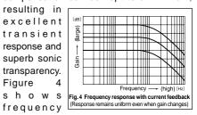
response for different gain settings of the current feedback amplifier. The graphs demonstrate that response remains uniform over a wide range.
