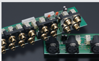
Gold-plated input/output jacks connected directly to relays
