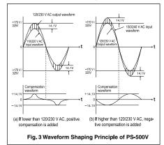
if the input is 130 V (240 V), 10 volts must be subtracted to yield 120 V (230 V), as shown in Figure 3 (b). In actual operation, the peak value of 10 V, namely 14.1 V is added or subtracted.
