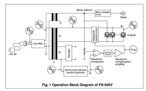
itself does not generate any high-frequency noise Figure 1 shows a block diagram of the unit. The signal from the secondary winding S1 of the transformer reaches the adding/subtracting circuit and appears at the output as output voltage (eo). A part of the output voltage is routed to the input of the waveform comparator for waveform comparison. The
