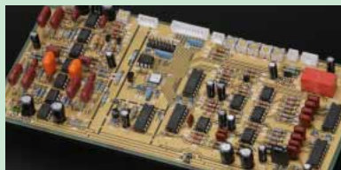
■ Assembly with reference signal generator and other circuitry
