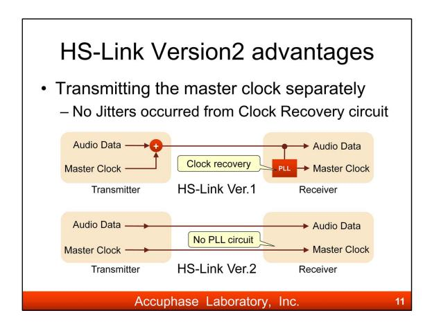
The biggest feature of HS-Link Ver.2 is sending the music signal and the master clock separately to D/A converter in a receiver.
