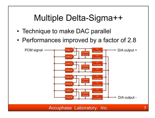
MDS++ is a technique to make DACs parallel. The same digital signal is supplied to each converter. The output of each DAC is combined.
