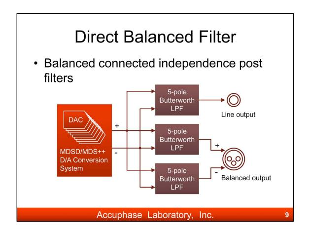
Full-balanced structure is employed after D/A converter section in DC-950.
