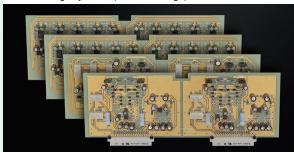
AAVA uses a unit amplifier configuration comprising the input buffer, 16 V-I amplifiers and current switches, current summing circuit, I-V converter amplifier, etc. Left and right channel circuitry is kept separate on each board.
