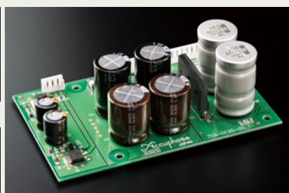
④ Low noise power supply circuits
