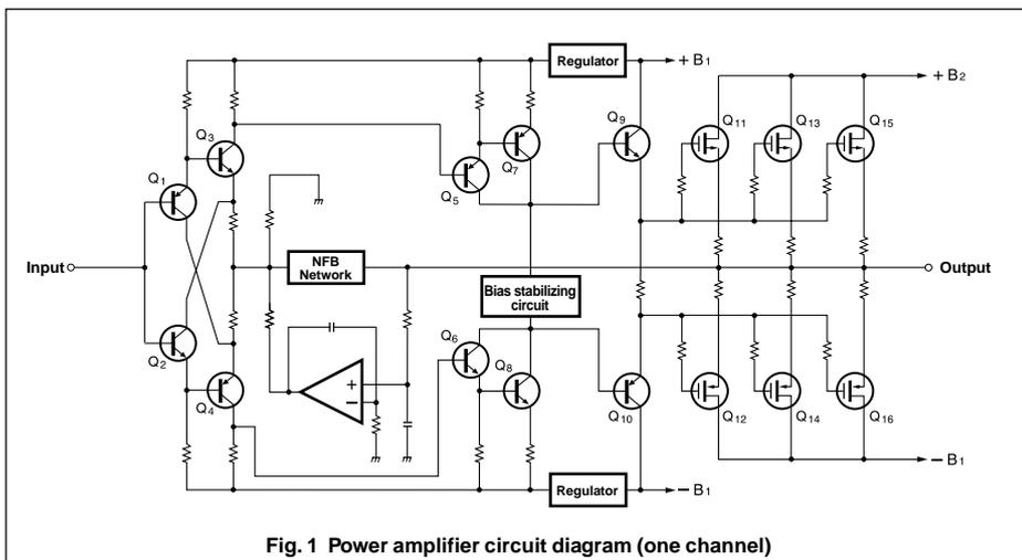
Fig. 1 Power amplifier circuit diagram (one channel)
