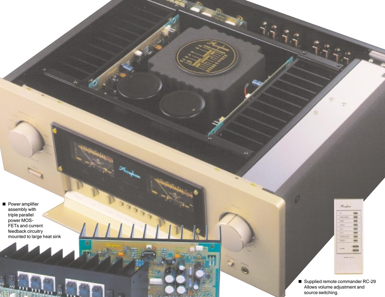
■ Power amplifier assembly with triple parallel power MOS-FETs and current feedback circuitry mounted to large heat sink
