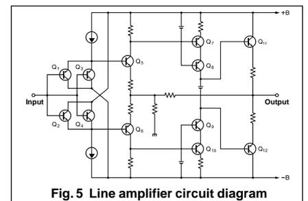
Fig. 5 Line amplifier circuit diagram
