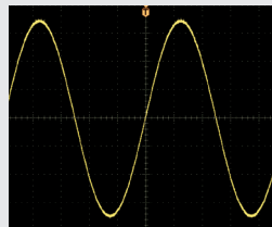
Photo (c) PS-1220 output waveform (distortion approx. 0.06%)
