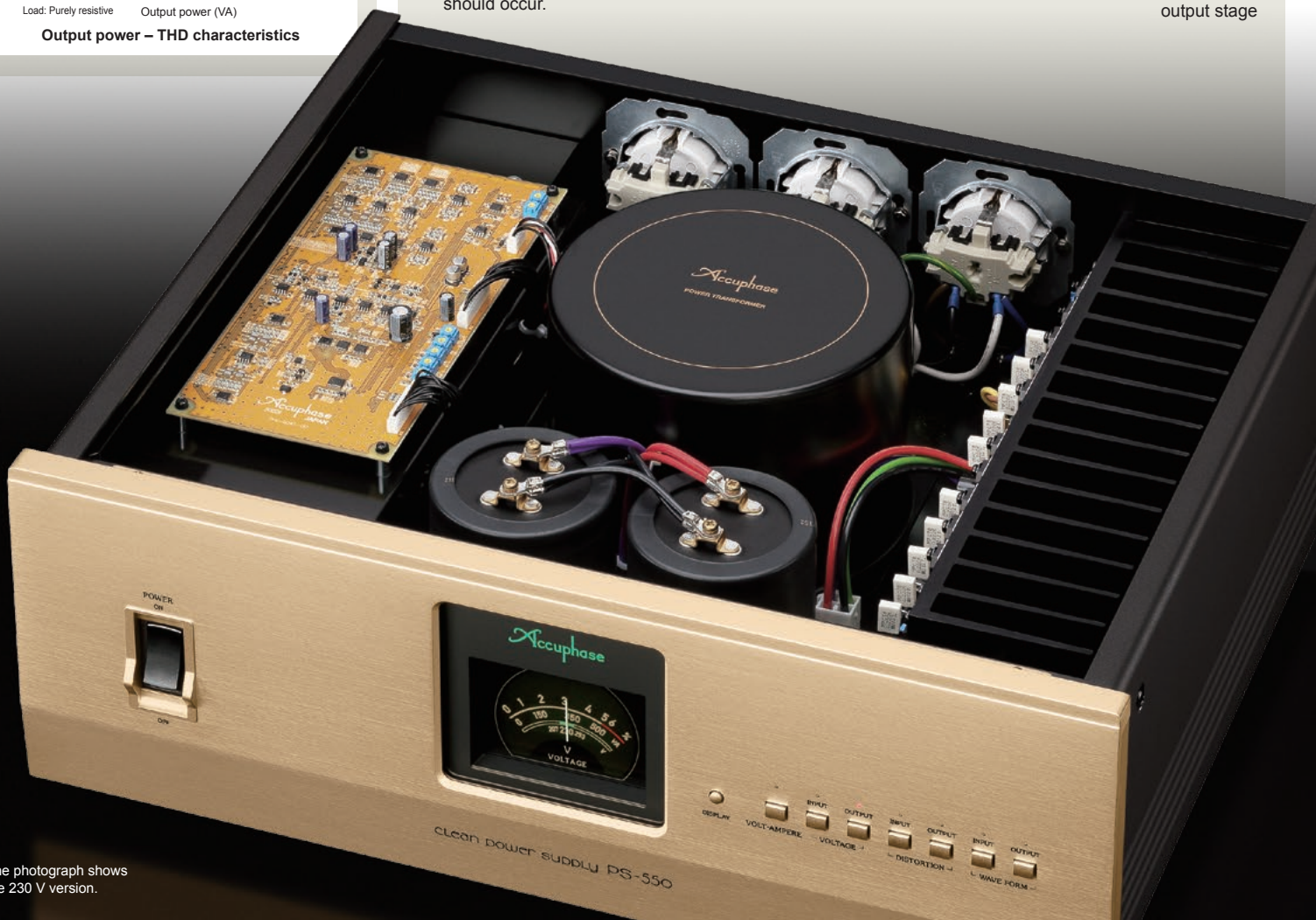
10-parallel push-pull output stage
