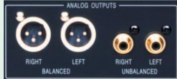
Balanced and unbalanced analog output connectors
