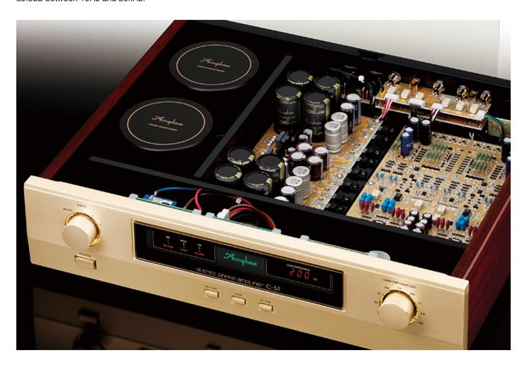
The C-57 features a dual mono circuit configuration and has a completely separate stabilised power supply and amplification circuits to minimise the effects of internal and external noise. It has low flux leakage, high-capacity toroidal transformers with eight 15,000uF filtering capacitors.
