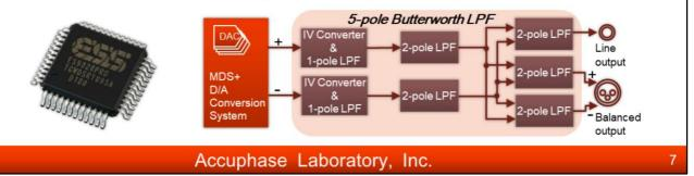
For D/A converter section, Accuphase updates the DAC chip to ESS Technology's 32bit Hyper Stream II DAC ES9026PRO for DP-450.
