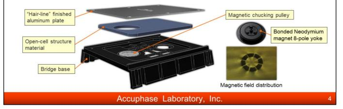
The newly-developed CD drive mechanism makes the bridge cover larger than former model, and applied threelayer structure with the open-cell structure material which absorbs the operational vibrations and noises.
