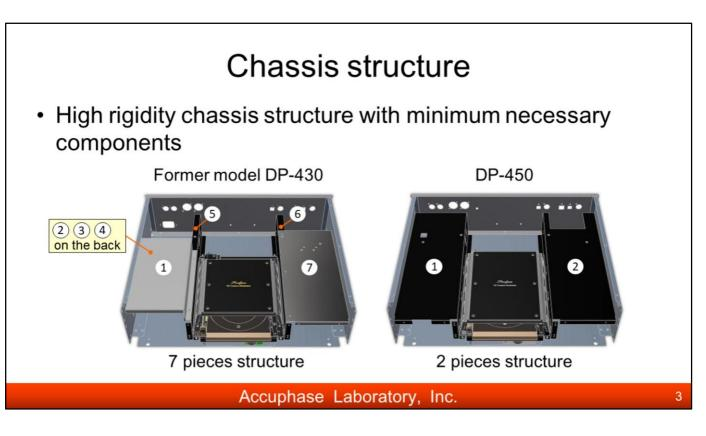
The strong integrated chassis structure that supports the CD drive mechanism adopts the 2 pieces structure, from the 7 pieces in the former DP-430.
