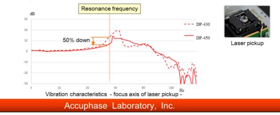
Thanks to the newly-developed CD drive mechanism, the DP-450 succeeds in 50% (6dB) reducing the external vibrations from being transmitted to the laser pickup at the resonance frequency.
