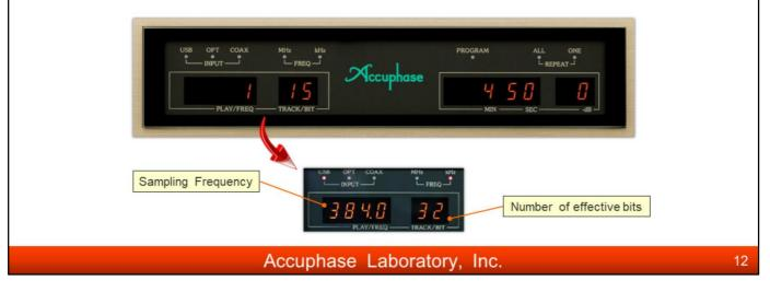
DP-450 can show the sampling frequency and the number of effective bits of all input signals on the front display.
