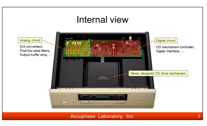
DP-450 is applied the systematic layout. Each circuit block is logically placed to make the signal path short as possible.
