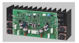
Power amplifier block with instrumentation amplifier configuration
