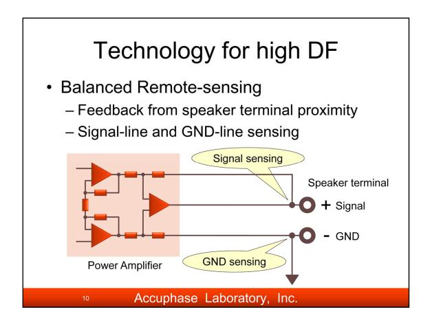
Remote-sensing is the technique to obtain lower output impedance of amplifier by negative feedback with signal sensing from close-up the speaker terminals.
