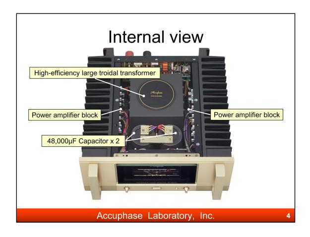
Strong power supply by large Troidal transformer with newly designed heat-radiation fins and a pair of 48,000µF capacitors are installed.
