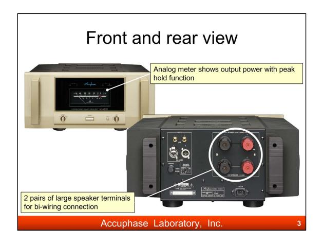
M-6200 has an analog power meter and it has peak-hold and hold time control function.
