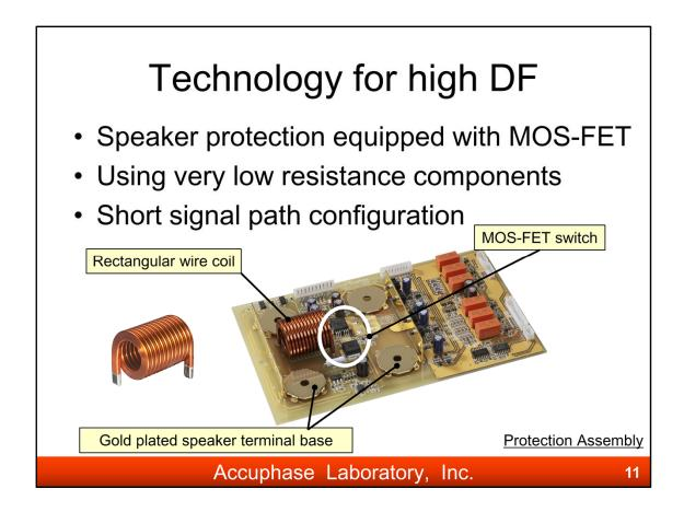
Mechanical relay is the most popular component for speaker protection. It does not have good reliability and low contact resistance either.
