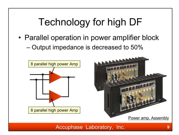
Output impedance is decreased by the multiple connected power amplifiers with 8-parallel push-pull arrangement of high power transistors.
