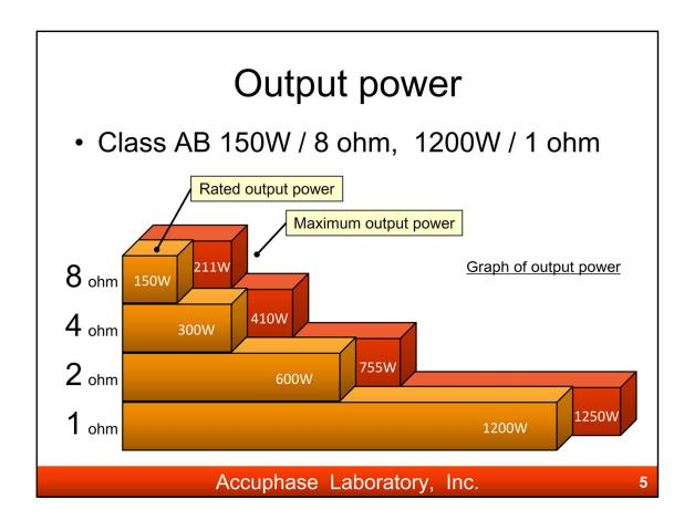
The continuous average output power is 150W into 8 ohm load.
