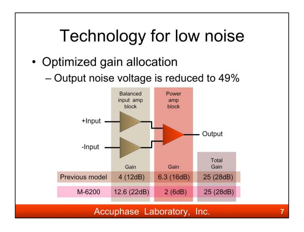
The output noise is reduced by some technologies. Optimizing gain allocation of 2 amplifier blocks which is constructed with instrumentation amplifier.
