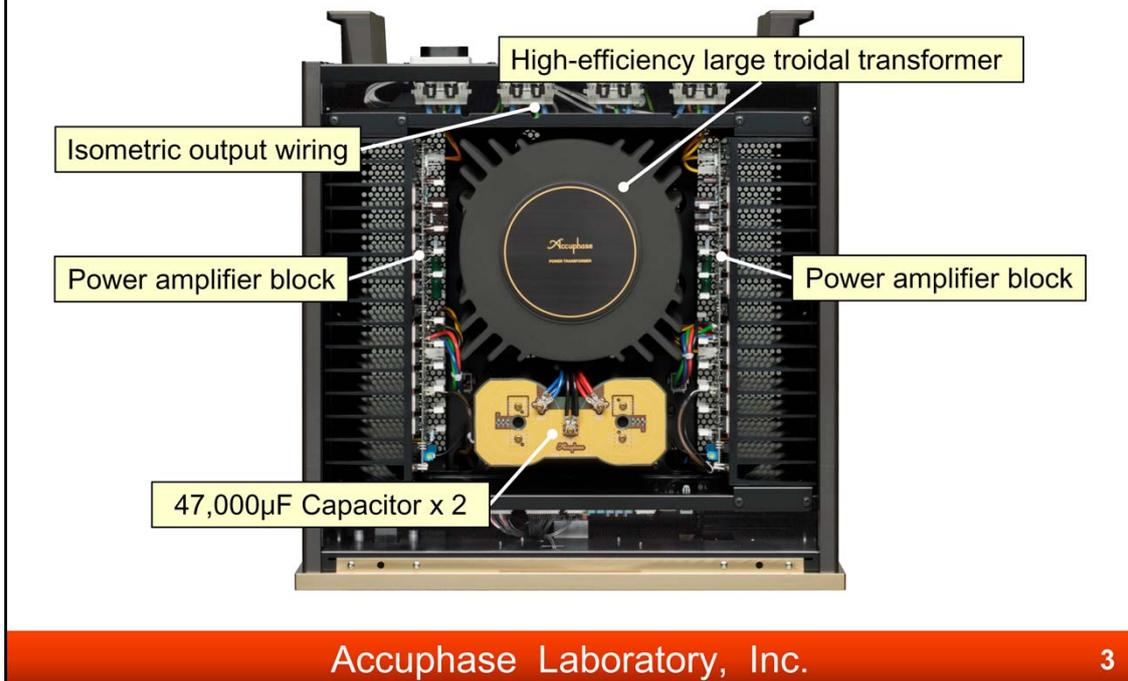
PS-1230 has a symmetric internal structure same as Accuphase stereo power amplifiers.
